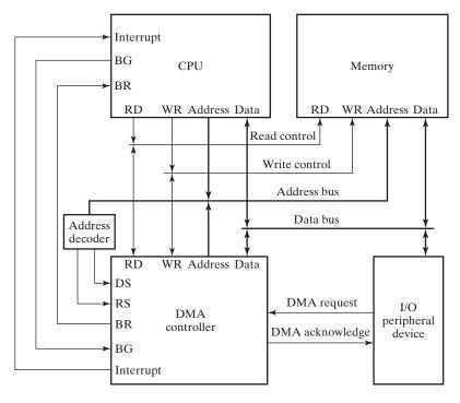
■ **FIGURE 11-20**DMA Transfer in a Computer System
