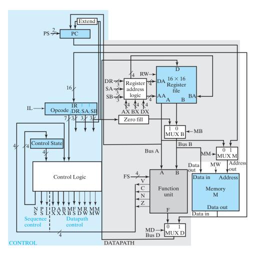
☐ **FIGURE 8-18**Block Diagram for a Multiple-Cycle Computer
