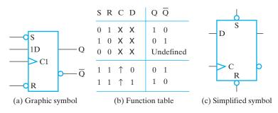
☐ **FIGURE 4-12**D Flip-Flop with Direct Set and Reset
