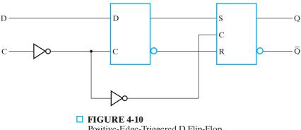
Positive-Edge-Triggered D Flip-Flop
