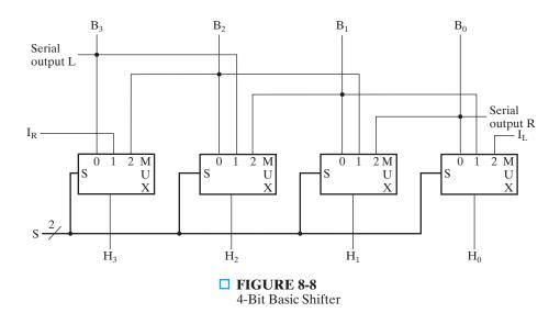
employed to specify what goes into  $I_R$  and  $I_L$  during a single bit-position shift. Note that to shift an operand by m > 1 bit positions, this shifter must perform a series of m 1-bit position shifts, taking m clock cycles.
