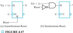
Asynchronous and Synchronous Reset for *D* Flip-flops
