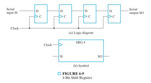
the next flip-flop. All flip-flops have a common clock-pulse input that activates the shift.
