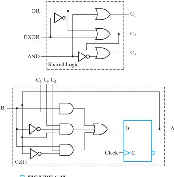
□ FIGURE 6-17 Logic Diagram—Register-Cell Design Example 6-1
