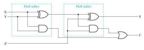
☐ FIGURE 3-42 Logic Diagram of Full Adder
