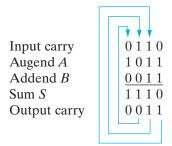
The input carry in the least significant position is 0. Each full adder receives the corresponding bits of A and B and the input carry, and generates the sum bit for S and the output carry. The output carry in each position is the input carry of the next-higher-order position, as indicated by the blue lines.
