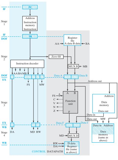
■ **FIGURE 10-4**Block Diagram of Pipelined Computer
