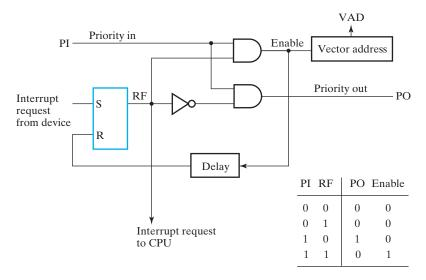
☐ **FIGURE 11-16**One Stage of the Daisy Chain Priority Arrangement
