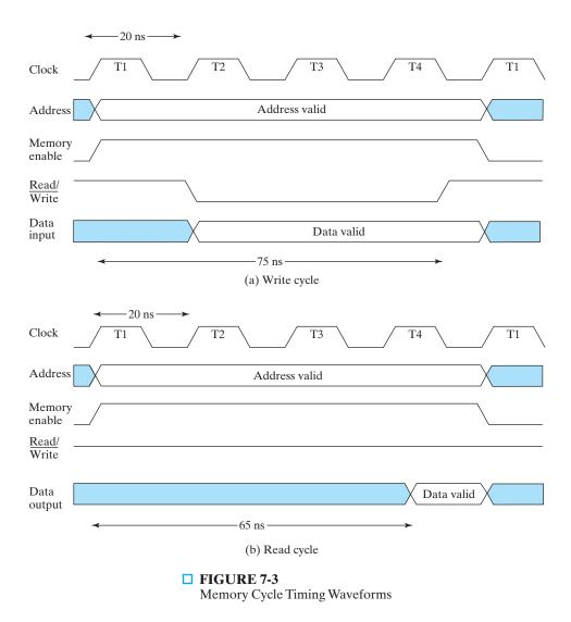
stable for a short time after the Read/Write goes to 1, again to avoid destroying data in other memory words. At the completion of the fourth clock pulse, the memory write operation has ended with 5 ns to spare, and the CPU can apply the address and control signals for another memory request with the next T1 pulse.
