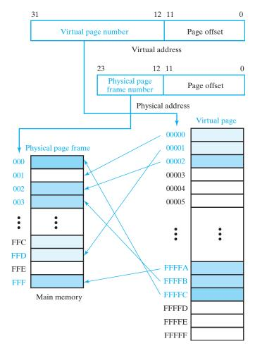
□ FIGURE 12-11 Virtual and Physical Address Fields and Mapping
