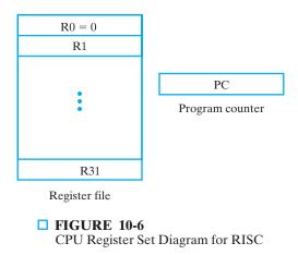
pipelines, these stores and loads require more than one clock cycle for their execution. To prevent these factors from degrading RISC performance, a larger register file is required.
