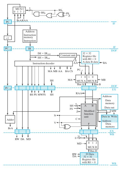
☐ **FIGURE 10-8**Pipelined RISC CPU
