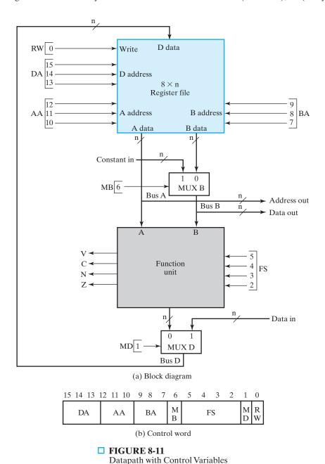
N (sign), and Z (zero). MUX D selects the function unit output or the data on *Data in* as input for the register file.
