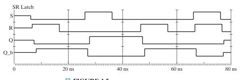
☐ **FIGURE 4-5**Logic Simulation of *SR* Latch Behavior
