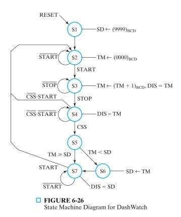
state becomes S7. If TM is greater than or equal to SD, then SD is unchanged, and the state becomes S7. In state S7, the smallest dash time stored in SD is displayed until START is pushed to cause the state to change to S2, beginning the timing of another dash.
