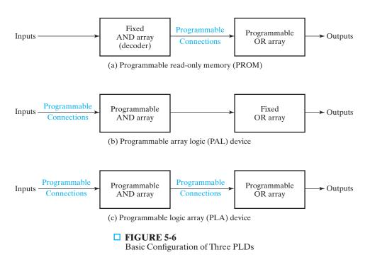
AND array may be shared by any OR gates to provide the required sum-of-products implementations. The names PLA and PAL® emerged for devices from different vendors during the development of PLDs.
