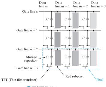
☐ **FIGURE 11-4** Liquid Crystal Subpixel Array voltages are inverted each time a row is written. When Gate Line 3 is returned to 0 volts, the transistor turns off and the voltage is stored on capacitance C. The rows of the LCD are successively written one at a time, with a full panel write taking less than a sixtieth of a second.
