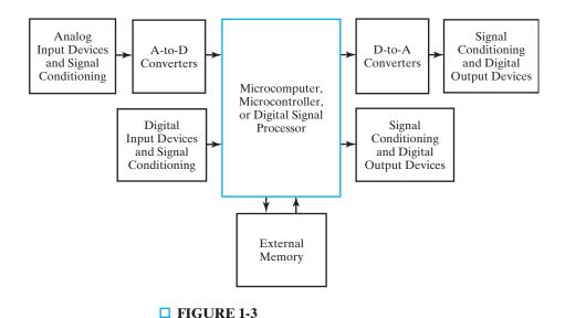
Block Diagram of an Embedded System
