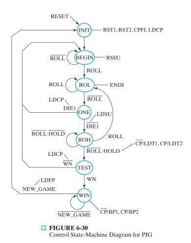
from Table 6-18 replace the output actions and status-based input conditions in Figure 6-29 to form the state diagram in Figure 6-30.
