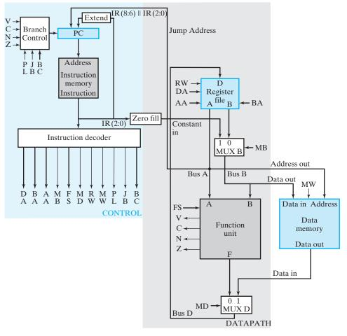
☐ **FIGURE 8-15**Block Diagram for a Single-Cycle Computer
