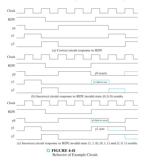
are all invalid states and give an incorrect output sequence. Thus, the circuit has again failed. Whether or not these failures occur depends upon circuit delays, the setup and hold times, and the detailed behavior of the flip-flops. Since none of these can be tightly controlled, we need a solution to prevent these failures that is independent of these parameters. Such a solution is the use of a synchronizing flip-flop.
