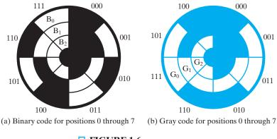
■ **FIGURE 1-6**Optical Shaft-Angle Encoder
