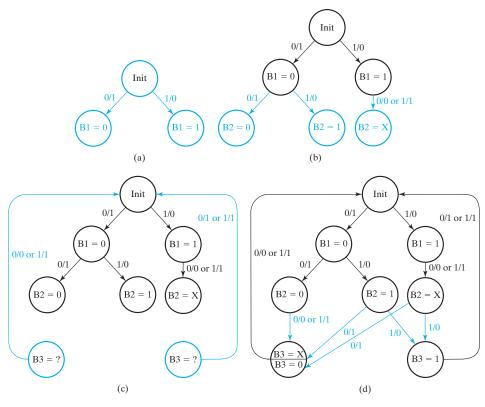
☐ **FIGURE 4-19**Construction of a State Diagram for Example 4-4
