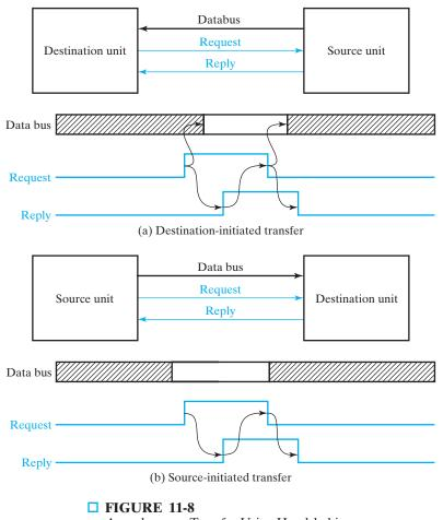
Asynchronous Transfer Using Handshaking
