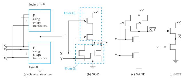
☐ **FIGURE 5-3**Fully Complementary CMOS Gate Structure and Examples
