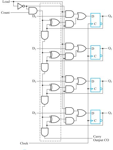
■ **FIGURE 6-14**4-Bit Binary Counter with Parallel Load
