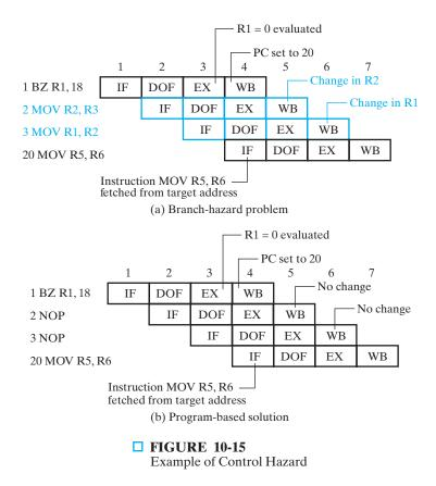
*PC* is set to 20 on the clock edge at the end of cycle 3. But the MOVA instructions in locations 2 and 3 are into the EX and DOF stages, respectively, after the clock edge. Thus, unless corrective action is taken, these instructions will complete execution, even though the programmer's intention was for them to be skipped. This situation is one form of a *control hazard*.
