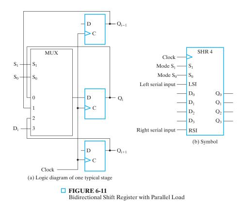
The "No Change" operation is implicit if none of the conditions for transfers is satisfied. When the mode control  $S_1S_0=00$ , input 0 of the multiplexer is selected. This forms a path from the output of each flip-flop into its own input. The next clock transition transfers the current stored value back into each flip-flop, and no change of state occurs. When  $S_1S_0=01$ , the terminal marked 1 on the multiplexer
