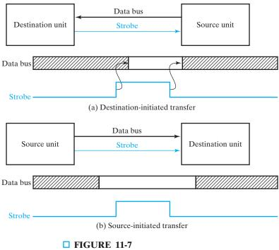
Asynchronous Transfer Using Strobing
