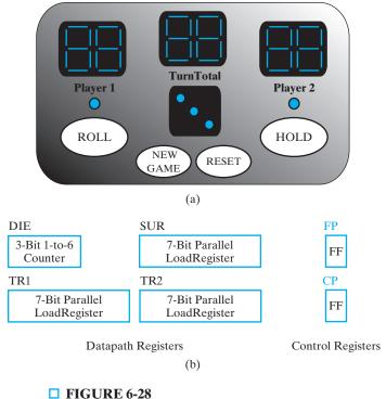
PIG: (a) Exterior View of PIG, (b) PIG Registers
