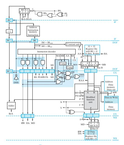
■ **FIGURE 10-12**Pipelined RISC: Data Hazard Stall
