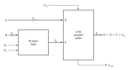
☐ **FIGURE 8-3**Block Diagram of an Arithmetic Circuit
