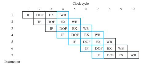
☐ **FIGURE 10-5**Pipeline Execution Pattern of Register Number Program
