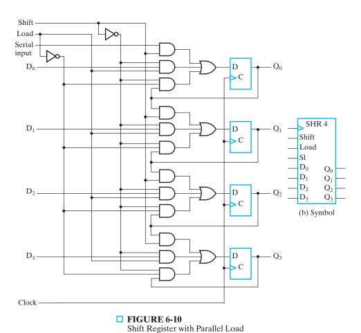
The operation of this register is specified in Table 6-6 and is also given by the register transfers:
