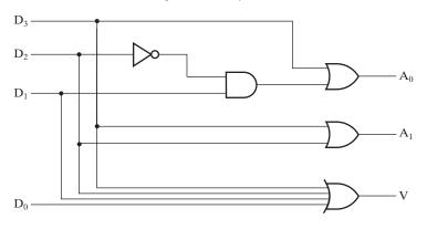
☐ FIGURE 3-23 Logic Diagram of a 4-Input Priority Encoder
