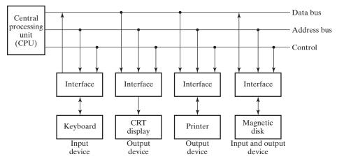
■ **FIGURE 11-5**Connection of I/O Devices to CPU
