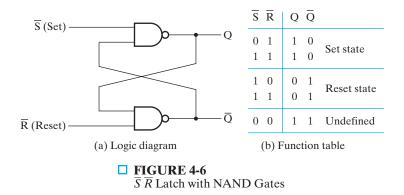
the NAND latch requires a 0 signal to change its state, it is referred to as an  $\overline{S}$   $\overline{R}$  latch. The bar above the letters designates the fact that the inputs must be in their complement form in order to act upon the circuit state.
