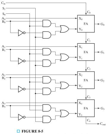
Logic Diagram of a 4-Bit Arithmetic Circuit
