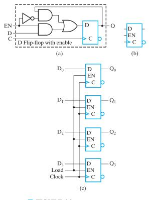
■ FIGURE 6-2 4-Bit Register with Parallel Load
