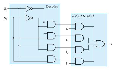
□ FIGURE 3-25 A Single-Bit 4-to-1-Line Multiplexer
