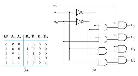
■ **FIGURE 3-16**A 2–to–4-Line Decoder with Enable
