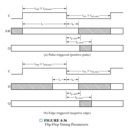
minimum and maximum values. Since the changes of the flip-flop outputs are to be separated from the control by the flip-flop inputs, the minimum propagation delay time should be longer than the hold time for correct operation. These and other parameters are specified in manufacturers' data books for specific integrated circuit products.
