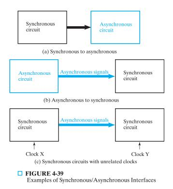
clock Y. Both of these cases can cause circuit malfunction, so we offer the synchronizing of such signals as a solution. In line with the perverse nature of asynchronous behavior, this solution isn't perfect, but suffers from a troublesome phenomenon referred to as metastability, a topic treated briefly here.
