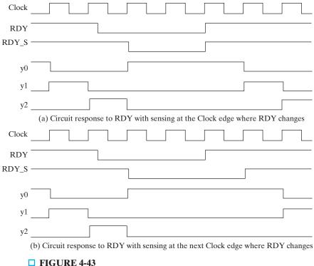
Behavior of Example Circuit with Synchronizing Flip-flop on RDY
