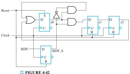
Example Circuit with Synchronizing D Flip-flop Added
