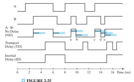
Examples of Behavior of Transport and Inertial Delays
