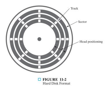
each sector is addressed using a single integer, with sectors numbered sequentially. The mapping from this address to the physical address is typically accomplished in the drive controller or drive electronics.
