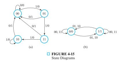
information as the state table and is obtained directly from it. The binary number inside each circle identifies the state of the flip-flops. For Mealy model circuits, the directed lines are labeled with two binary numbers separated by a slash. The input value during the present state precedes the slash, and the value following the slash gives the output value during the present state with the given input applied. For
