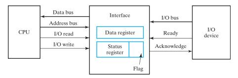
☐ **FIGURE 11-13**Data Transfer from I/O Device to CPU
