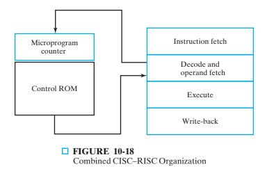
memory accesses in sequence, the decode stage produces a microcode address for the microcode ROM and replaces the usual decoder outputs with control values from the microcode ROM. Execution of microinstructions from the ROM, selected by the microprogram counter, continues until the execution of the instruction is completed.
