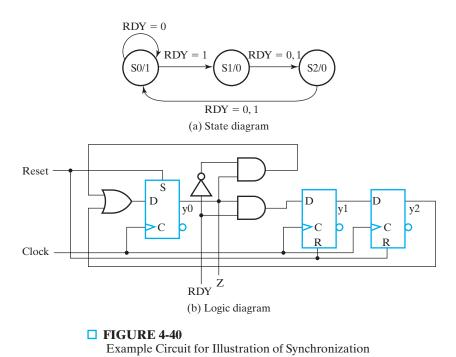
RDY = 0, then the circuit waits in state S0 until RDY = 1 causes it to go to state S1. Also, the state can change from S1 to S2 and from S2 to S0 with RDY = 0. All other combinations of state variables are invalid during the normal operation of the circuit.
