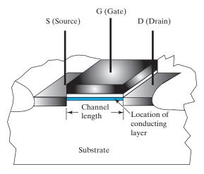
(a) Transistor geometry
