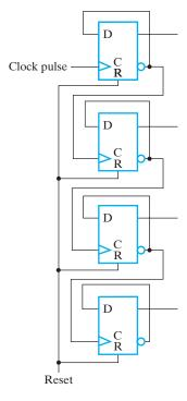
☐ **FIGURE 6-12** 4-Bit Ripple Counter
