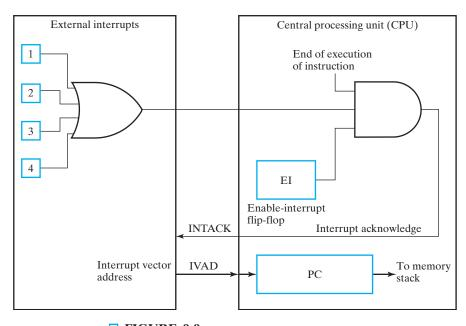
■ **FIGURE 9-9**Example of External Interrupt Configuration
