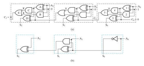
■ **FIGURE 3-52**Contraction of Adder to Incrementer
