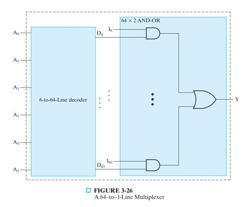
reduction to 3-input ANDs cannot be performed without replicating the output ANDs of the decoders. As a result, in almost all cases, the original structure has a lower gate-input cost. The next example illustrates the expansion to a multiple-bit multiplexer.
