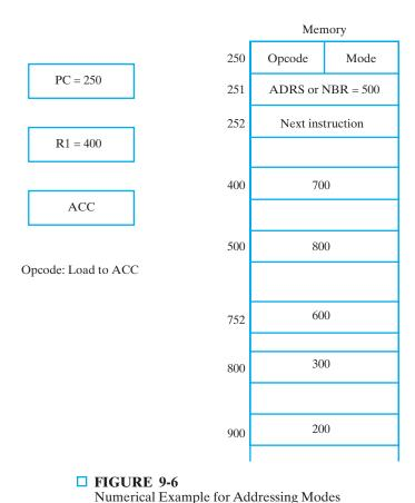
more compact instructions, since the relative address can be specified with fewer bits than are required to designate the entire memory address. This permits the relative address field to be included in the same instruction word as the opcode.
