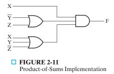
The gate structure of the product-of-sums expression consists of a group of OR gates for the sum terms (except for a single literal term), followed by an AND gate. This is shown in Figure 2-11 for the preceding function *F*. As with the sum of products, this standard type of expression results in a two-level gating structure.
