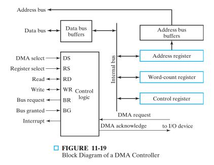
through the DMA request and DMA acknowledge lines by a prescribed handshaking procedure.
